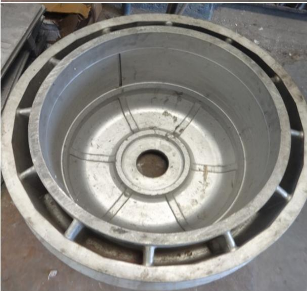
Item: Fan Hub (Indian Railway) Diameter 700mm X Height 500 mm Weight : 130 Kgs. Supplying to : Railways
