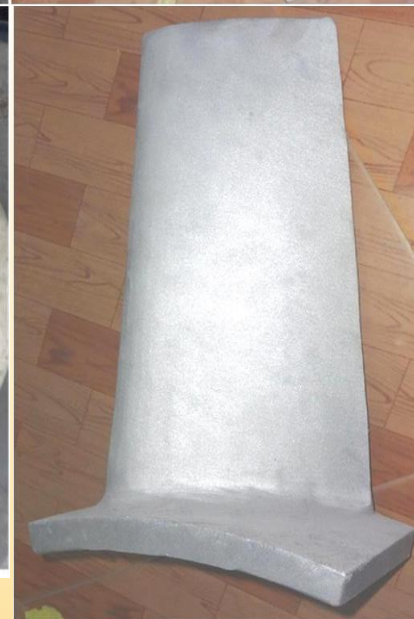
Item: Fan Blade Length 600mmx width 300mm Weight : 130 kgs. Supplying to : Railways
